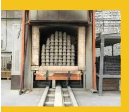
Fire assaying is the main method for defining most of the precious metals, the main stages of which are crucible or scorifying melting, cupelling. The success of the assaying significantly depends on the properties and quality of the assay labware.
